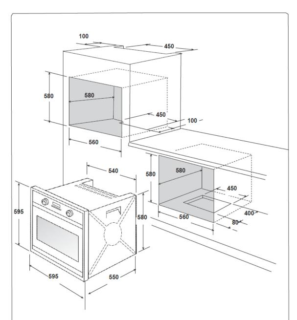
Cabinetry materials must be suitable to withstand temperatures up to 90°C
